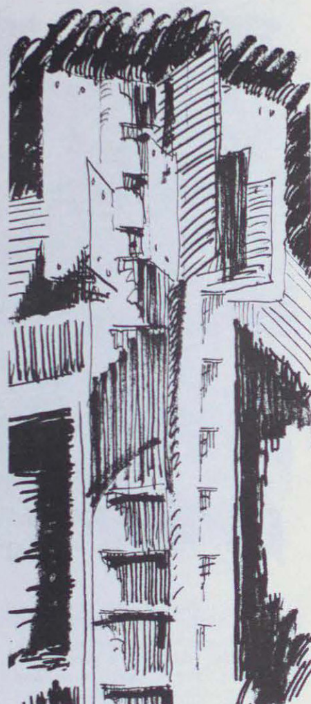
Noto Laundry: column with joining plates for future expansion.
