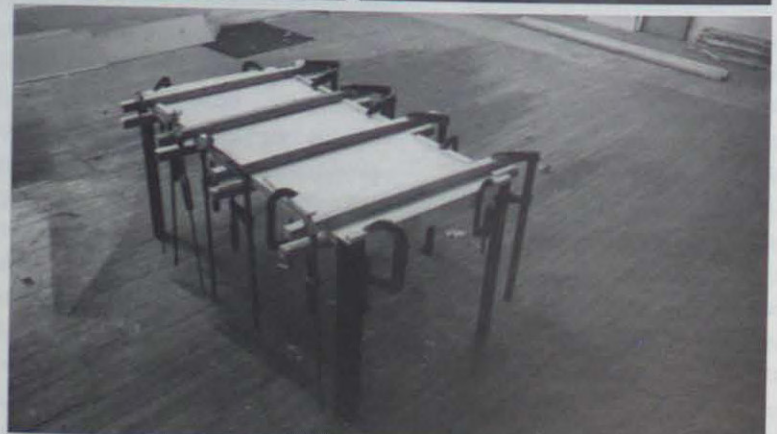
clamped with cauls - prototype 2
